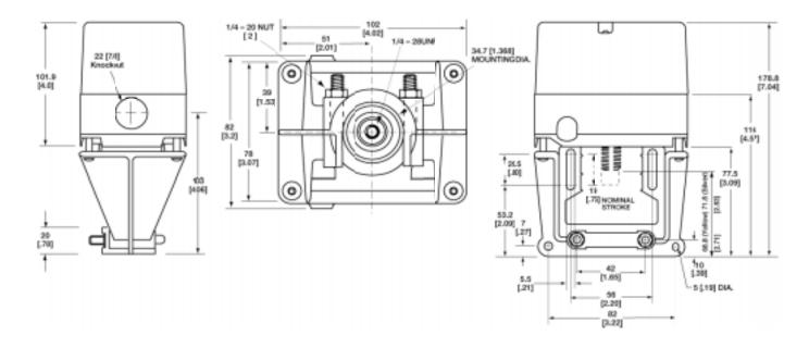
FIG. 1 -- DIMENSIONS OF ML7984 VALVE ACTUATOR IN MM (INCHES).
